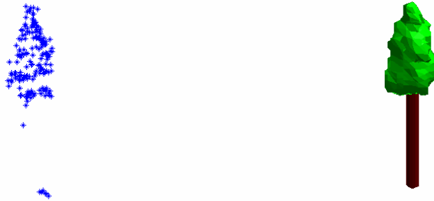
Figure 3. Visualization of the wrapped surface for a single tree. The single stand LIDAR point is shown in the left and the wrapped surface from the LIDAR points is shown in the right.
